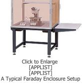
Experiments in electrophysiology, confocal microscopy, and other sensitive applications often need to be shielded from external interference from electrostatic fields and electromagnetic waves generated by AM/FM radio, CRT oscilloscopes, fluorescent lights, and other common lab equipment. Thorlabs' ScienceDesk™ Faraday Enclosure consists of a taut copper mesh that protects against these external sources of interference.
